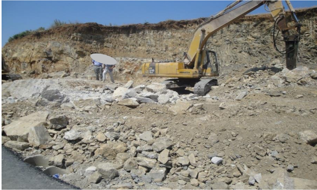
Figure 28 Damage to environment and risking the final bench as mining without criterion - ICMM
