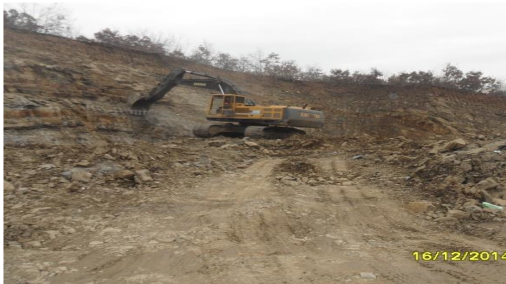
Figure 49 Mining without criterion, creation of altitude of benches and lack of recultivation - MESP
