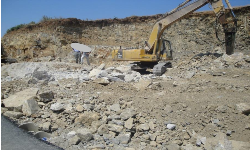
Figure 76 Damage to environment and risking the final bench as mining without criterion - Municipal inspectorate
