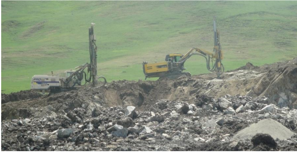
Figure 13 Preparation activity of a field for blasting - ICMM
