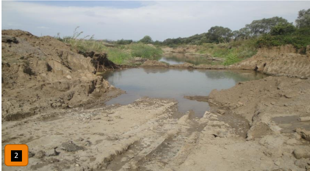
Figure 24 Water dump from mining of clay and sand, degrading basins and risk for people - ICMM
