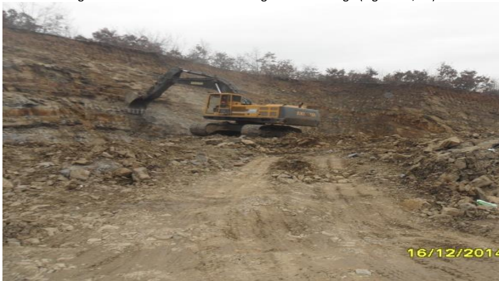
Figure 74 Mining without criterion, creation of altitude of benches and lack of recultivation- Municipal inspectorate
